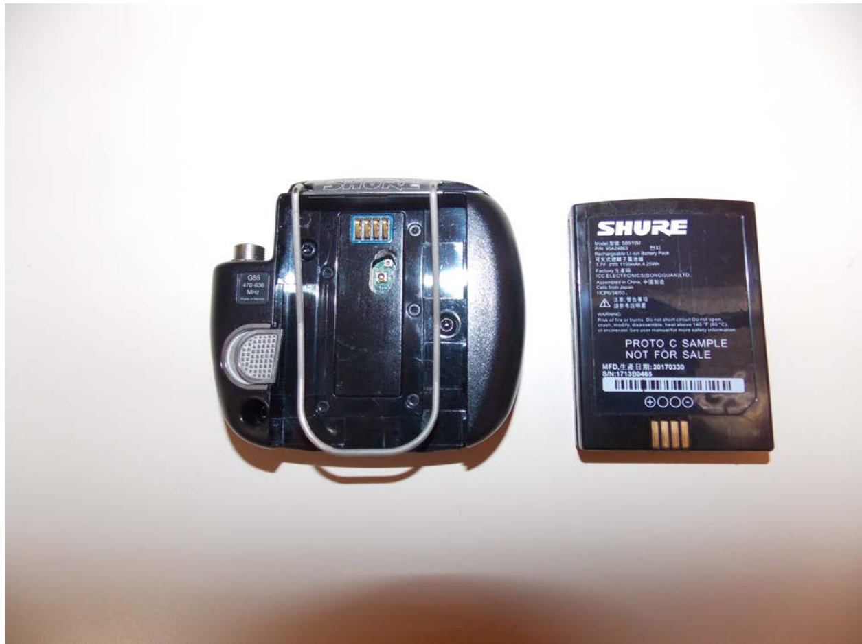
Back of Device with Li-Ion Battery
