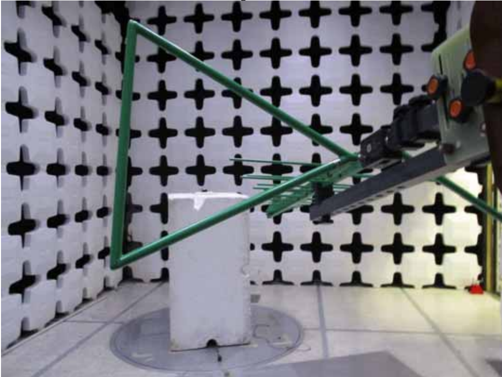
Test Setup for Radiated Emissions, 25MHz to 1GHz – Horizontal Polarization
