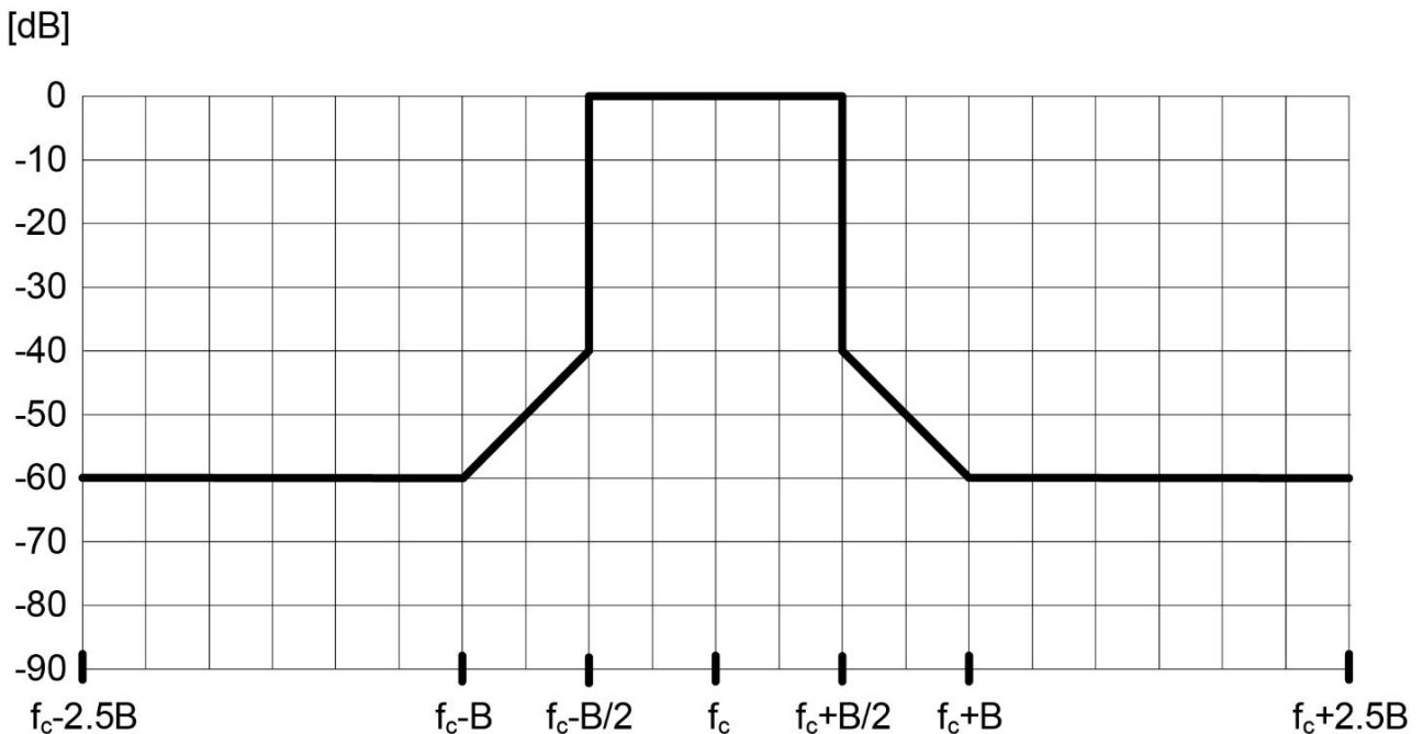
Figure 3: Transmit spectral power mask for WMAS, RBW = 100 kHz
