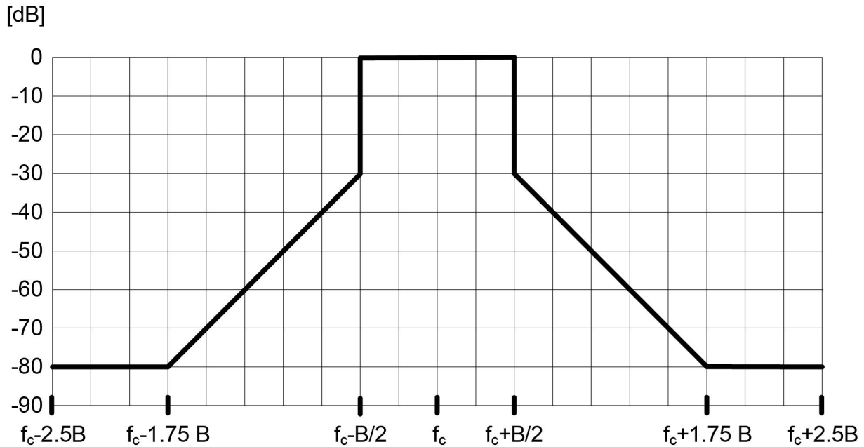
Figure 2: Transmit spectral power mask for equipment employing digital modulation, except WMAS, RBW = 1 kHz
