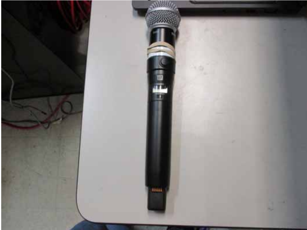
Photograph of the AD651B Talk Switch inserted in the ADX2FD Digitally Modulated Handheld Microphone
