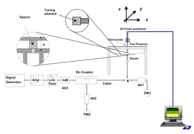
System Performance Check Setup Diagram
