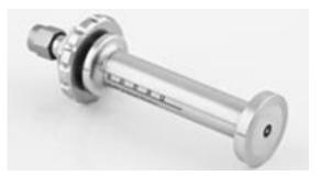
Evaluation of reference liquids over a broad frequency range for specific absorption rate (SAR) measurements, in accordance with IEC 62209, IEEE 1528, and several federal regulations. Evaluating Software: DAK software version 2.0
