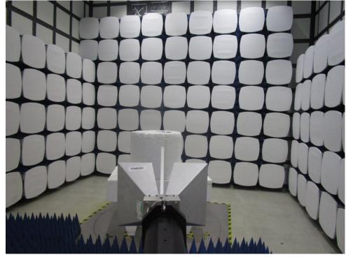
1.2 Radiated Spurious Emissions Test Setup
