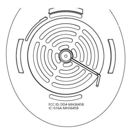
FCC ID and IC ID are underneath the earpad, the user can easily take off the earpad to see the IDs.
