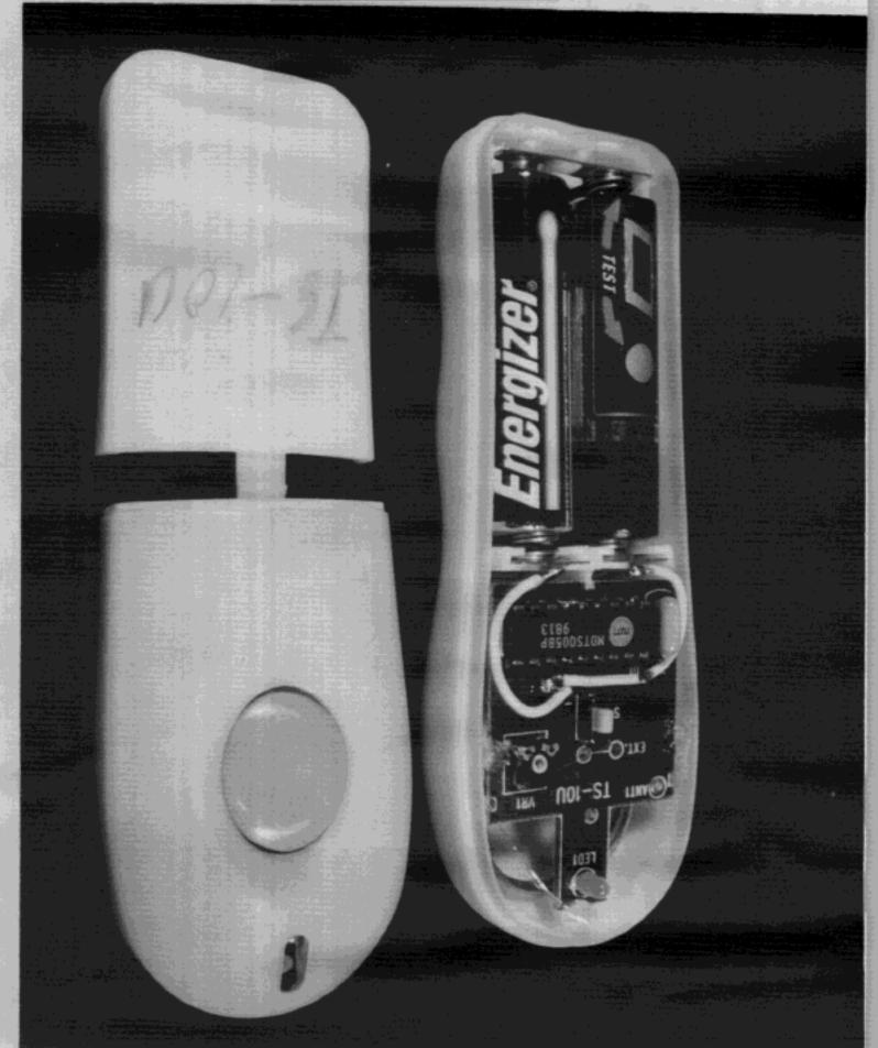
PHOTOGRAPH **04** FCC ID.:DC9TS-10U COMPONENT VIEW OF MAIN PCB
