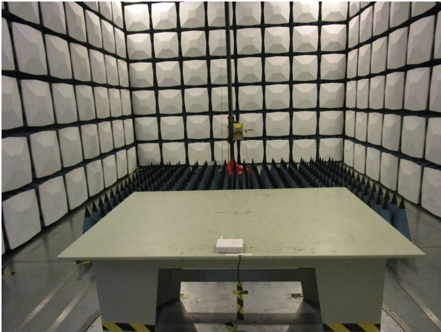
Radiated Emission- Rear View (Above 1GHz) (AC 12V)
