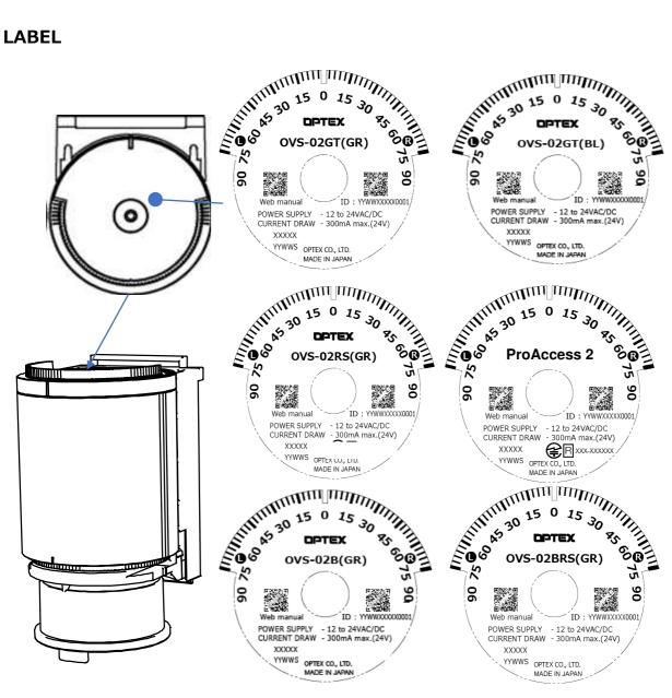
\*The label shown is permanently affixed and readily visible to the user. (Permanent adhesive of Acrylic adhesive is used.) The instoller can recognize this label when wiring. (Labeling requirement per 2.925)
