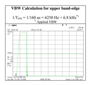
\* The transmitting time which occupied upper chirp frequency was applied for the VBW calculation.
