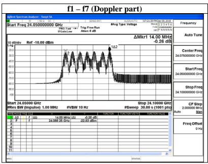
There are seven doppler frequencies and chirp part in one transmission period. These doppler parts and chirp part were compared to calculate the duty factor. The duty factor was calculated within doppler part, because doppler's dwell time is longer than the chirp part.
