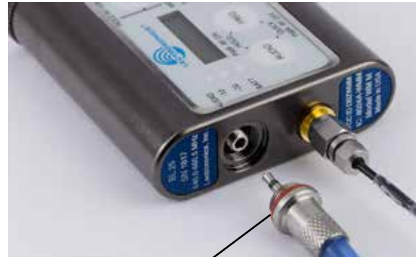
Treat O-ring with petroleum jelly before connecting (see page 11)
