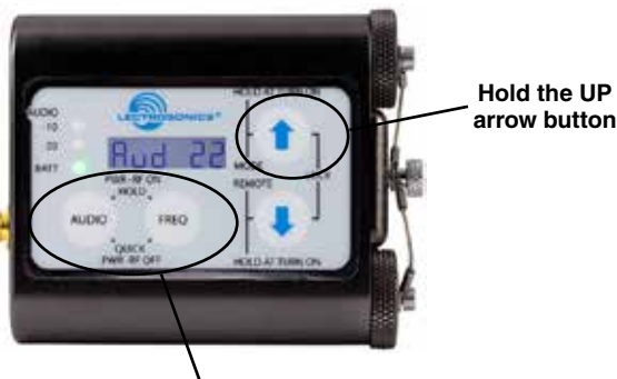
Then press the AUDIO and FREQ buttons at the same time
