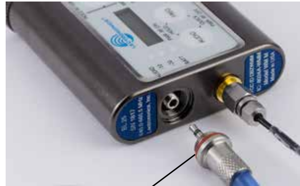
Treat O-ring with petroleum jelly before connecting (see page 11)
