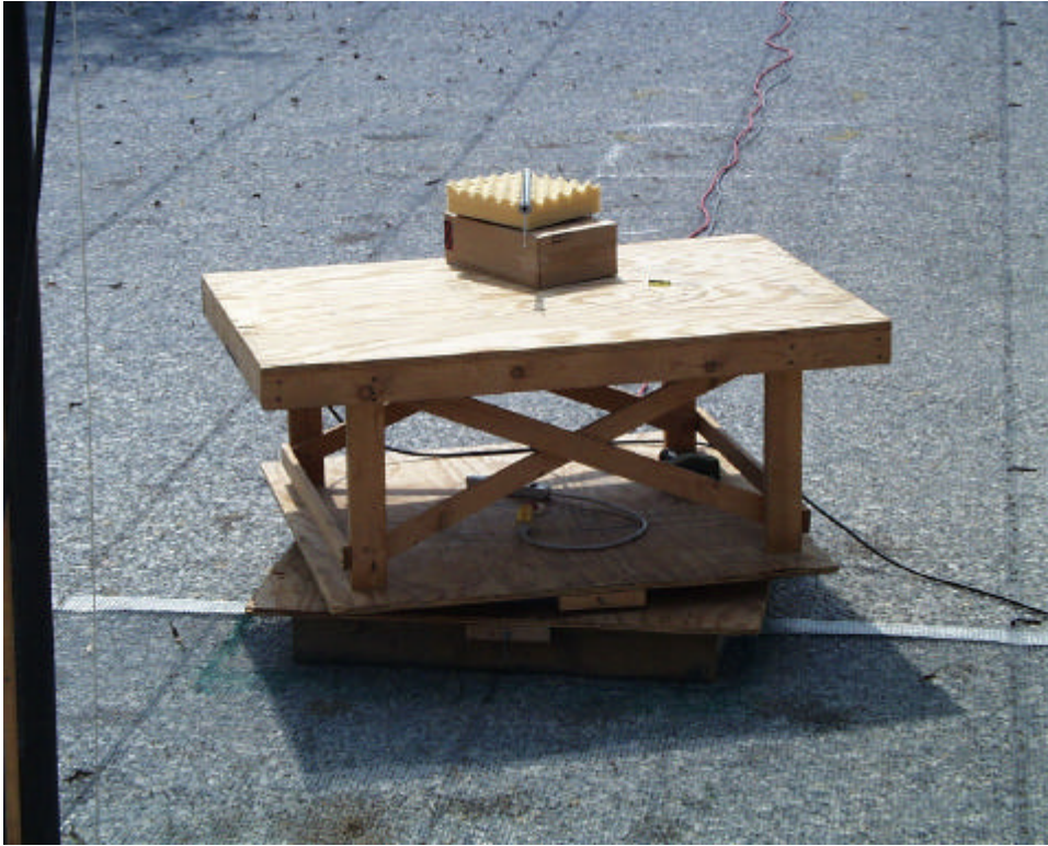
Photograph of substitution antenna setup at OATS.
