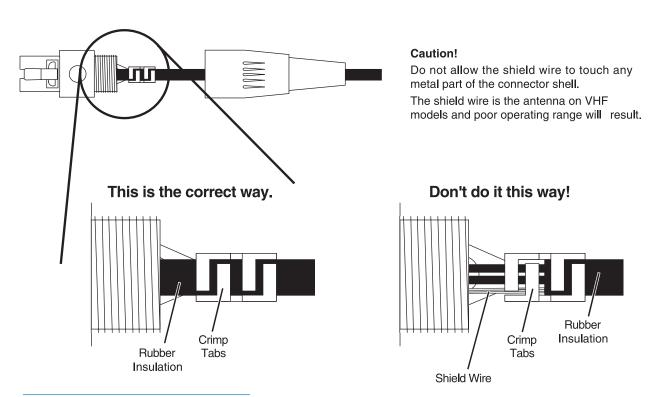
NOTE: This termination is required on VHF transmitters and will still work fine on UHF transmitters.
