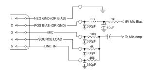
The best RF protection is accomplished by installing RF bypass capacitors at the mic capsule. If this is not possible, or if you are still having problems, capacitors can be installed on the mic pins inside the TA5F connector housing.
