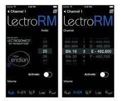
The iPhone version keeps each available setting on a separate page with the list of options for that setting. On iOS, the "Activate" toggle switch must be enabled to show the button which will then activate the tone. The iOS version's default orientation is upside-down but can be configured to orient right-side up. The purpose for this is to orient the phone's speaker, which is at the bottom of the device, closer to the transmitter microphone.
