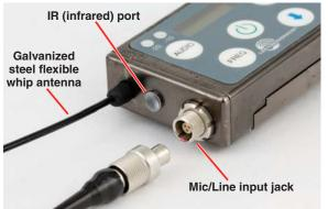
The antenna is a flexible whip made of galvanized steel, permanently attached to the transmitter to prevent damage from heavy use. The IR port is capped with a translucent dome material to broaden the reception angle. The input jack is a rugged 3-pin LEMO connector with a threaded locking sleeve.
