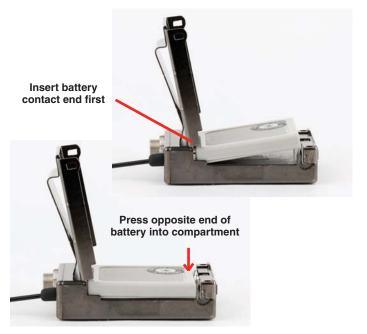
If the battery is inserted incorrectly, the door will close but the unit will not operate.
