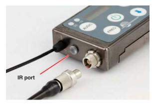
Place the transmitter close to the IR enabled receiver with the ports facing each other within a foot or two apart. Send the settings with the trigger on the receiver. If the settings are successfully transferred, a confirmation message will appear on the transmitter LCD.
