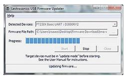
WARNING: Do not disrupt the microUSB cable during updating.
