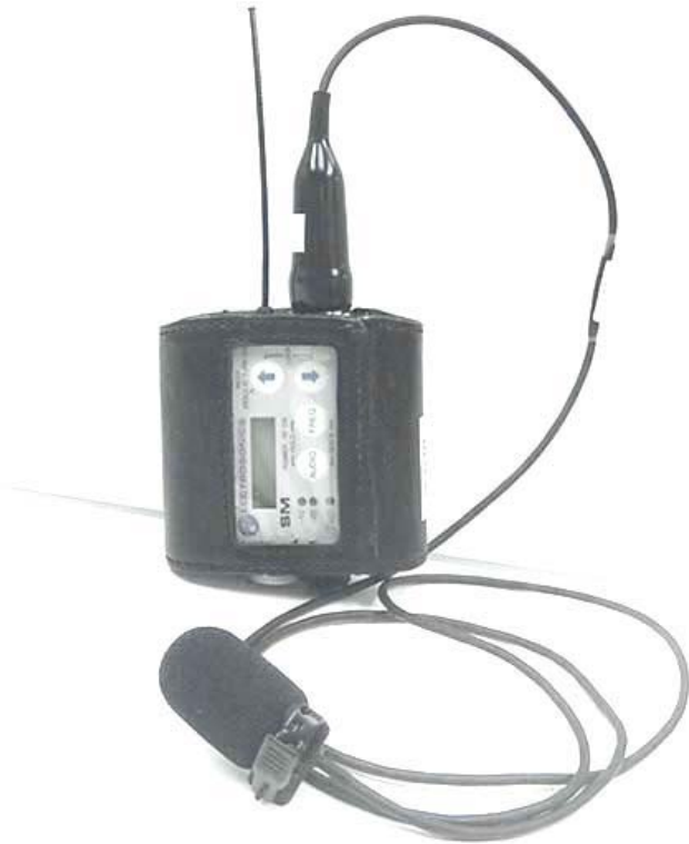
Front Side of DUT with Belt-Clip Holster and Electret Microphone Audio Accessory
