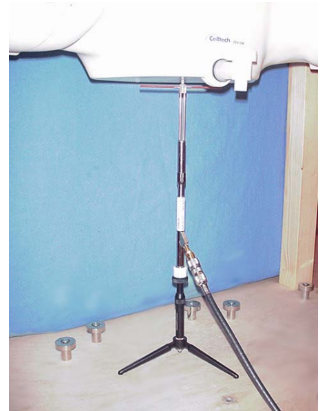
835MHz Dipole Setup
