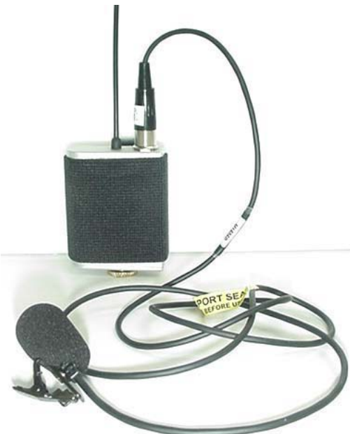
Front of Belt-Clip Holster with Microphone Front of DUT Facing Front of Holster
