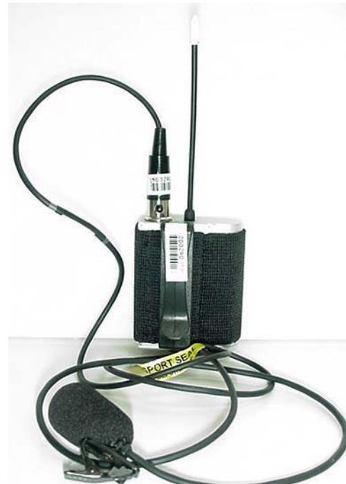
Back of Belt-Clip Holster with Microphone Front of DUT Facing Front of Holster
