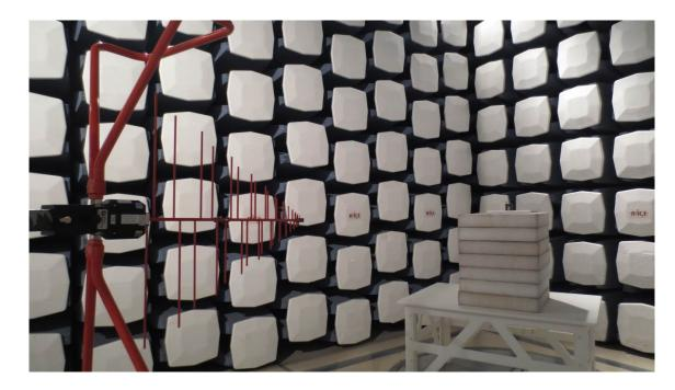
11.1 Radiated Spurious Emissions Below 1 GHz – Front View
