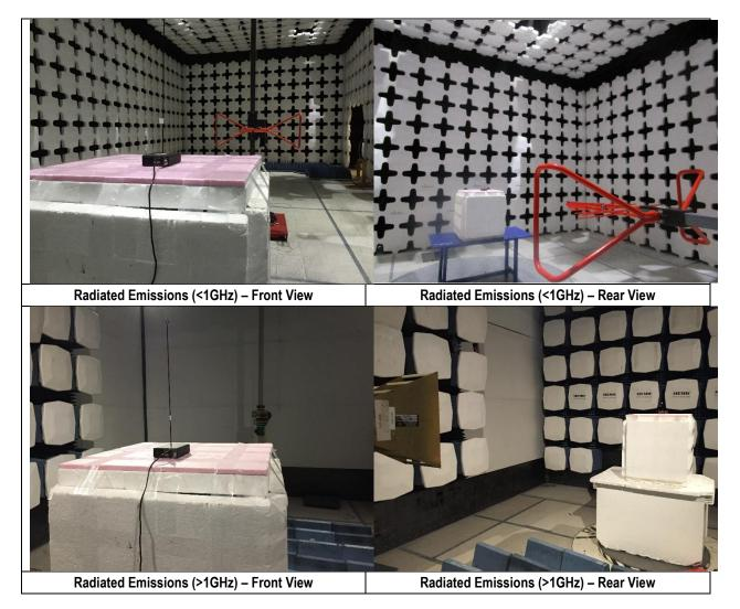
Note: The spurious emission in different EUT orientation was investigated, including the EUT standing up position and the laying down position. The EUT orientation shown in above setup photo is the worst case position.
