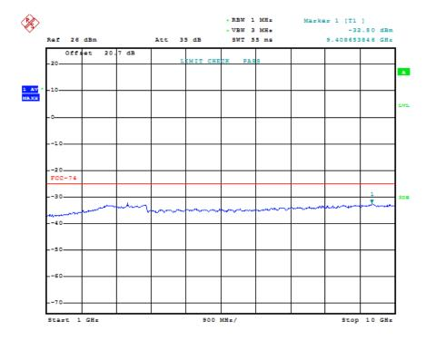
Note: The limit line in above plots is based on IC limit; however, FCC limit line is -13 dBm. Plots comply with both FCC and IC requirements
