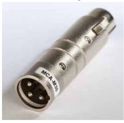
This adapter may be needed if you are experiencing noise or distortion with measurement microphones, particularly the Earthworks M30. The adapter has a common mode choke for suppressing RF noise. If your microphone signal exhibits the problems listed above when connected to a UH400, HM or DPR transmitter, insert the adapter between the microphone and the transmitter.
