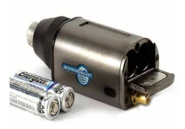
Batteries operate in series, with a connecting plate built into the battery door
