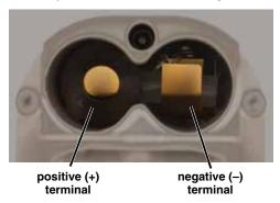
Note: It is possible to install the batteries backward and close the battery door, but the batteries will not make contact and the unit will not power up.
