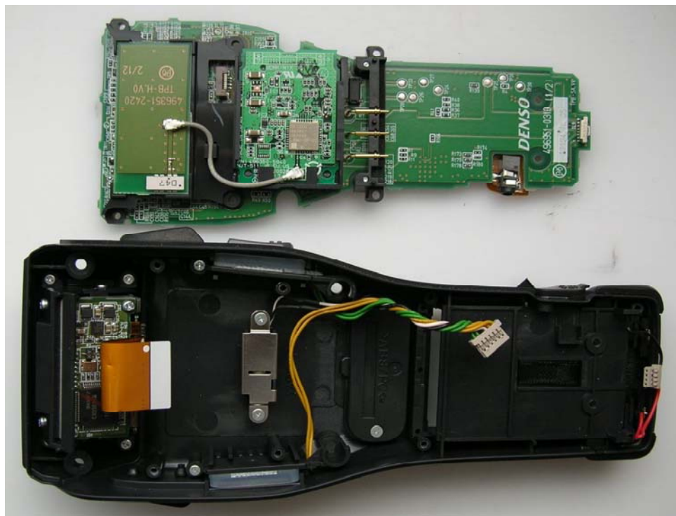
Assembling Wireless LAN Adapter assembled holder on main circuit of Barcode Handy Terminal.
