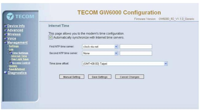
Figure 6-44-1. Management - Internet Time - Time Setting - NTP setting
