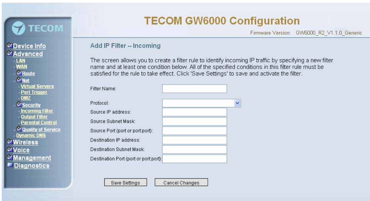
Figure 6-15-2. Advanced Setup – Security – Incoming IP Filtering – Add
