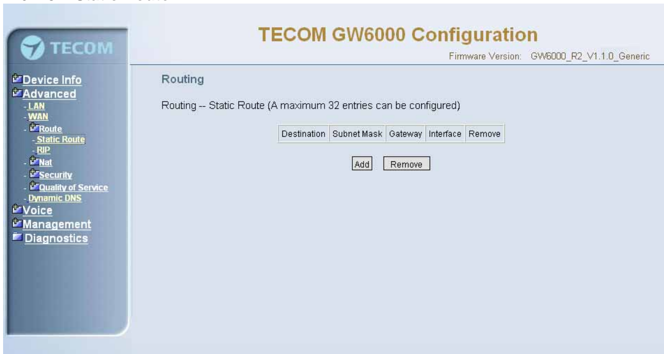
Figure 6-10-1. Advanced Setup – Route – Static Route
