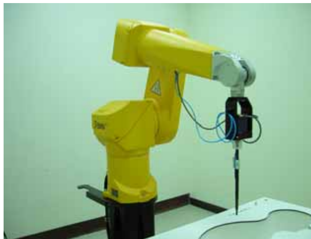
Fig. 5.2 Probe setup on robot
