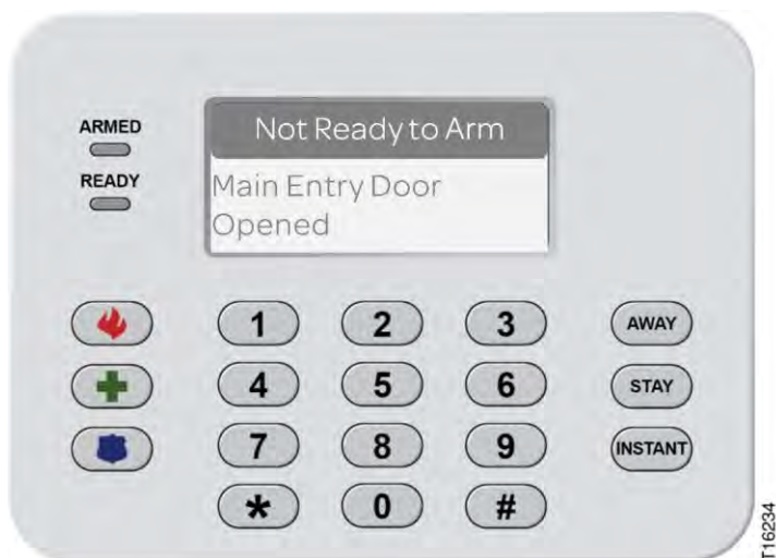
Figure 102: Keypad (Model SR-KPD02)—Open State Device(s)
