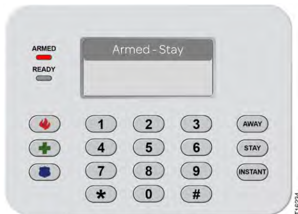
Figure 100: Keypad (Model SR-KPD02)—Armed – Stay Mode
