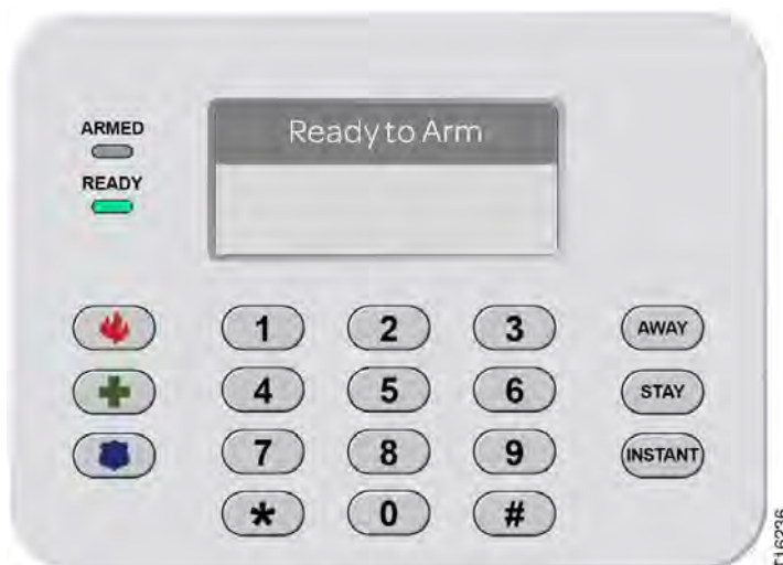
Figure 107: Keypad (Model SR-KPD02)—Ready to Arm
