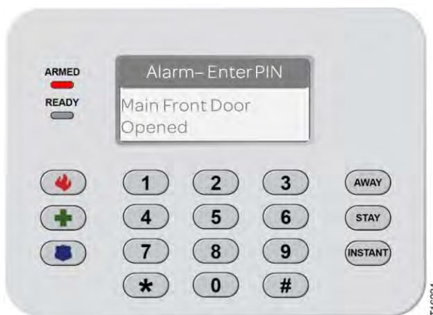
Figure 104: Keypad (Model SR-KPD02)—Entry Delay (Opened Devices)
