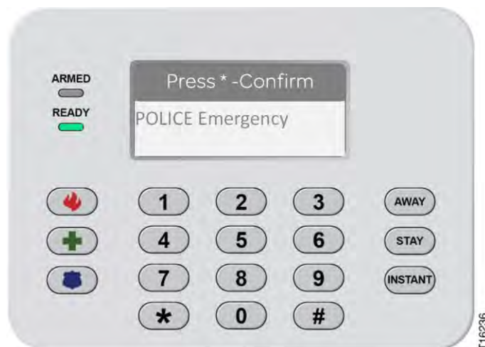
Figure 117: Keypad (Model SR-KPD02)—POLICE (Press * –Confirm)
