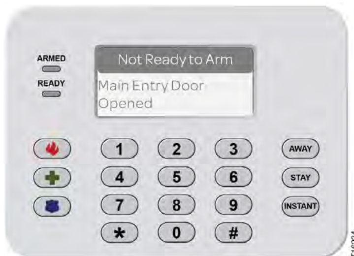
Figure 96: Keypad (Model SR-KPD02)—Not Ready to Arm
