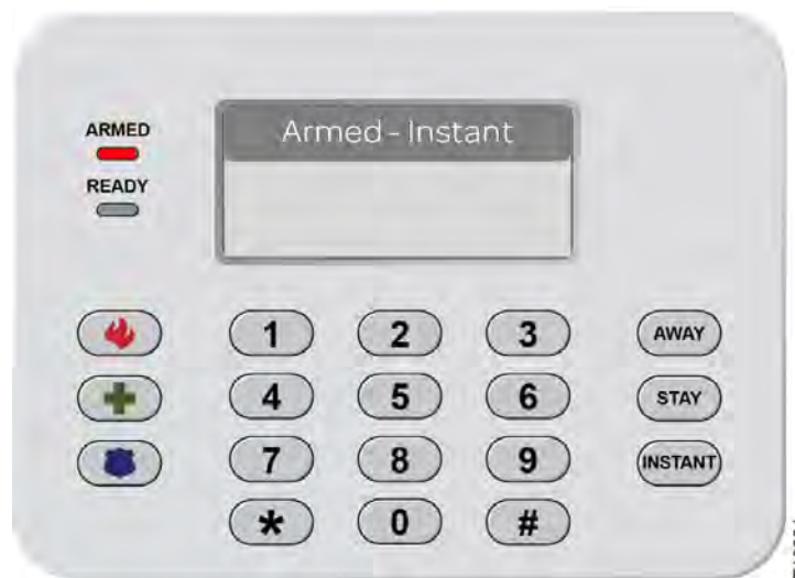
Figure 101: Keypad (Model SR-KPD02)—Armed - Instant
