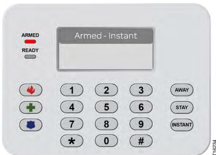
Figure 106: Keypad (Model SR-KPD02)—Armed - Instant
