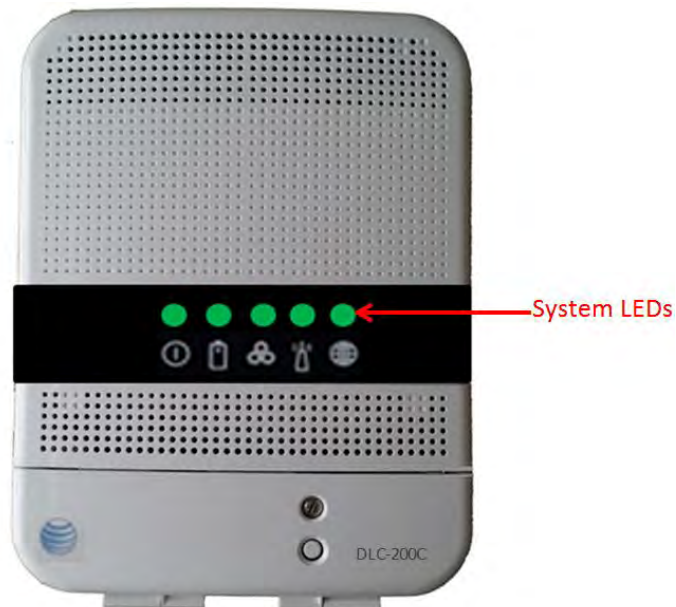
Figure 42: System LEDs Operational Indicators
