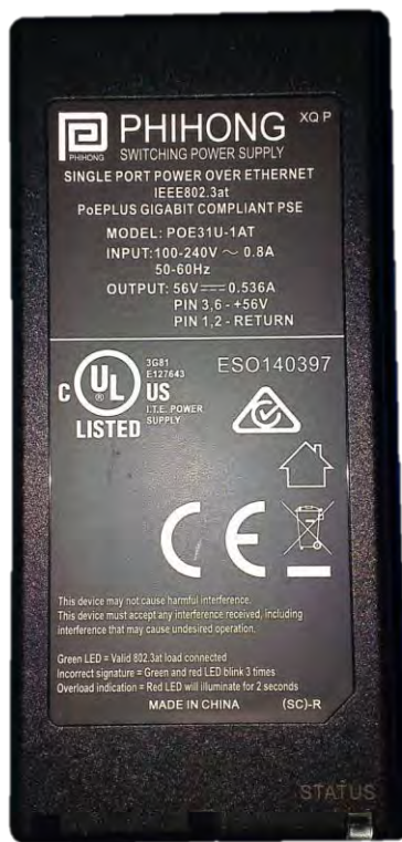
Figure 45: PHIHONG XQP POE31U-1AT PoE Front Panel
