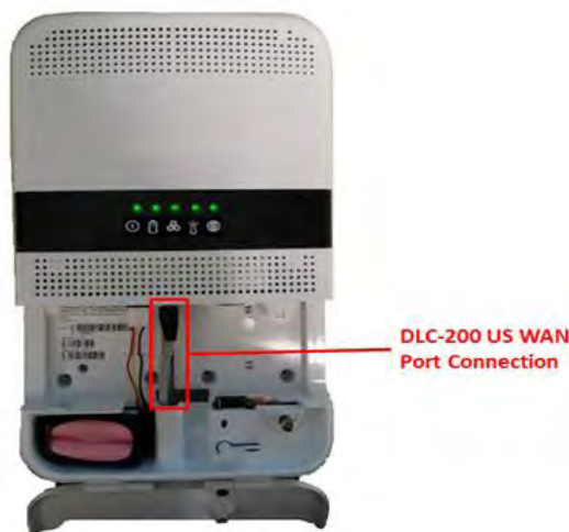
Figure 39: DLC-200C WAN Port Connection
