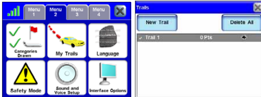
The My Trails button on Menu 2 (left figure) calls up the Trails Menu (right) where you can create, edit or delete trails.
