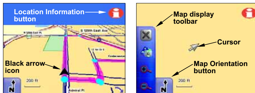
A black arrow icon (left) indicates your position on the map screen. The map screen with map display toolbar buttons is shown at right.
