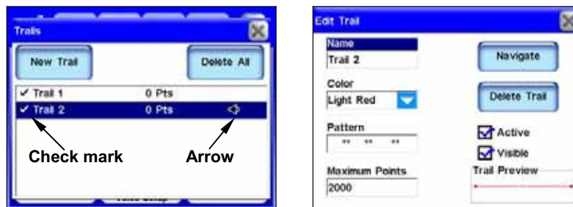
Trails Menu (left) with Trail 2 highlighted. Trail 2 is active, indicated by the arrow on the right. The Edit Trail screen (right) allows you to modify an existing Trail.
