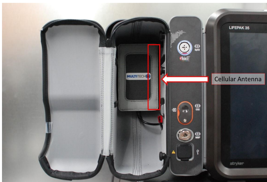
Photo 1-2 View of Cell Modem Inside Left Bag
