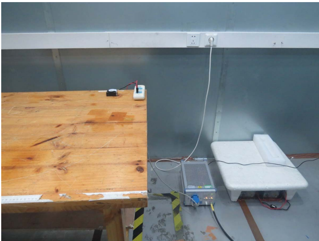
Picture 2 Conducted Emission Test Setup
