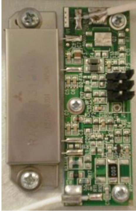
Board top side components. Bottom side no components, ground plane.
