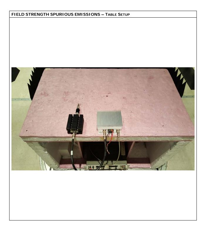
FIELD STRENGTH SPURIOUS EMISSIONS – 9 KHz – 30 MHz
