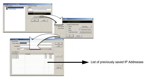
FIG. 17 Assigning Communication Settings and TCP/IP Settings
