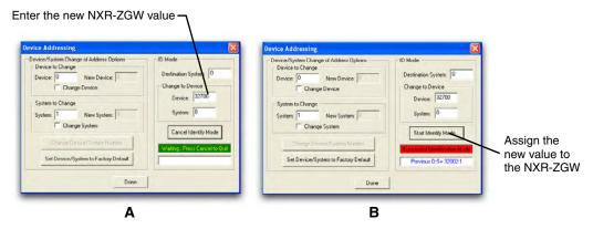
FIG. 19 Device Addressing dialog (using the ID mode to set the NXR-ZGW device value)
