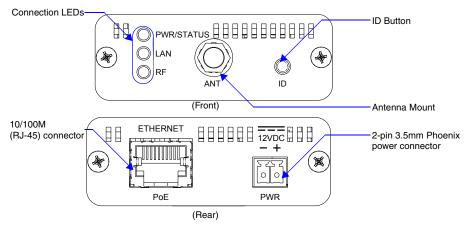
**FIG. 1** Front and Rear Components of the NXR-ZGW
