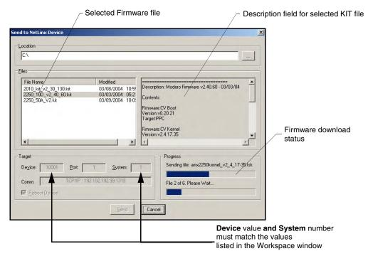
FIG. 18 Send to NetLinx Device dialog
