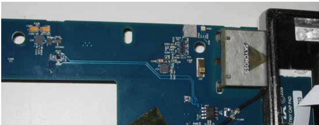
Integrated circuit board antenna (top) and Skycross antenna (bottom)
