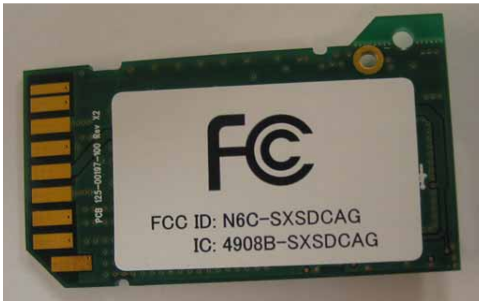
Top and Bottom of WiFi radio card used in the system
