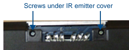
FIG. 101 Location of screws under IR emitter cover
