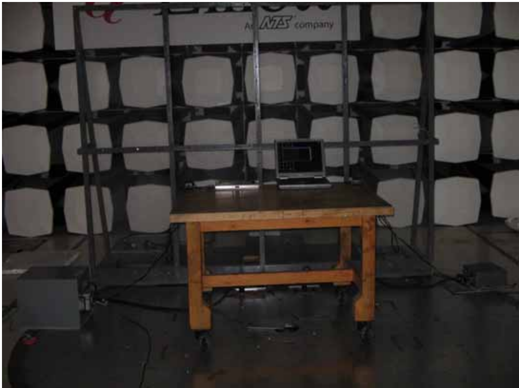
Test Configuration – AC Conducted Emissions
