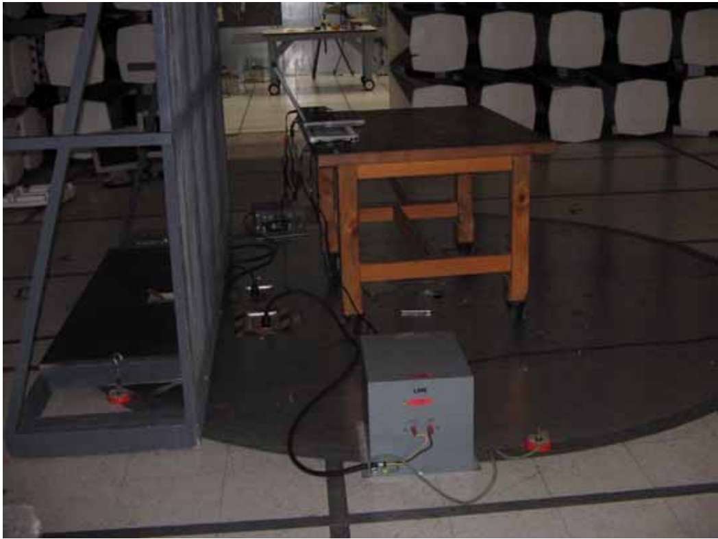
Test Configuration – AC Conducted Emissions
