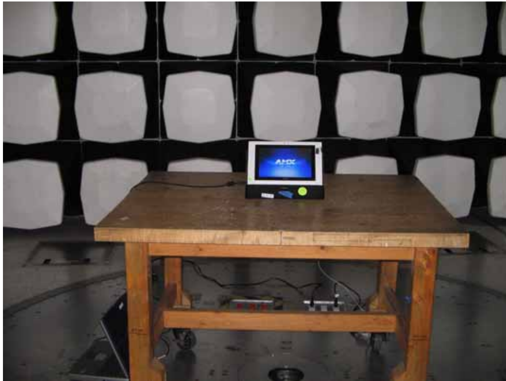
Radiated Emissions Test Configuration – System in the Table Docking Station
