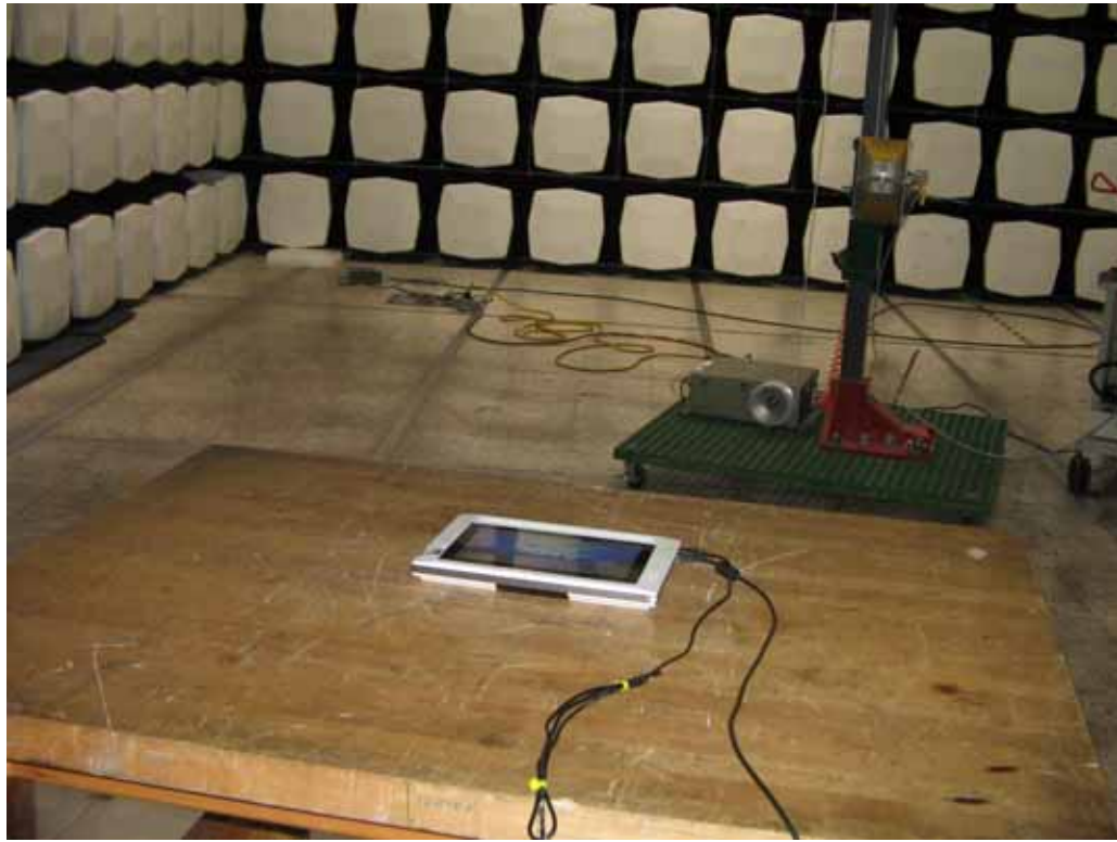
Radiated Emissions Test Configuration – System Stand-Alone
