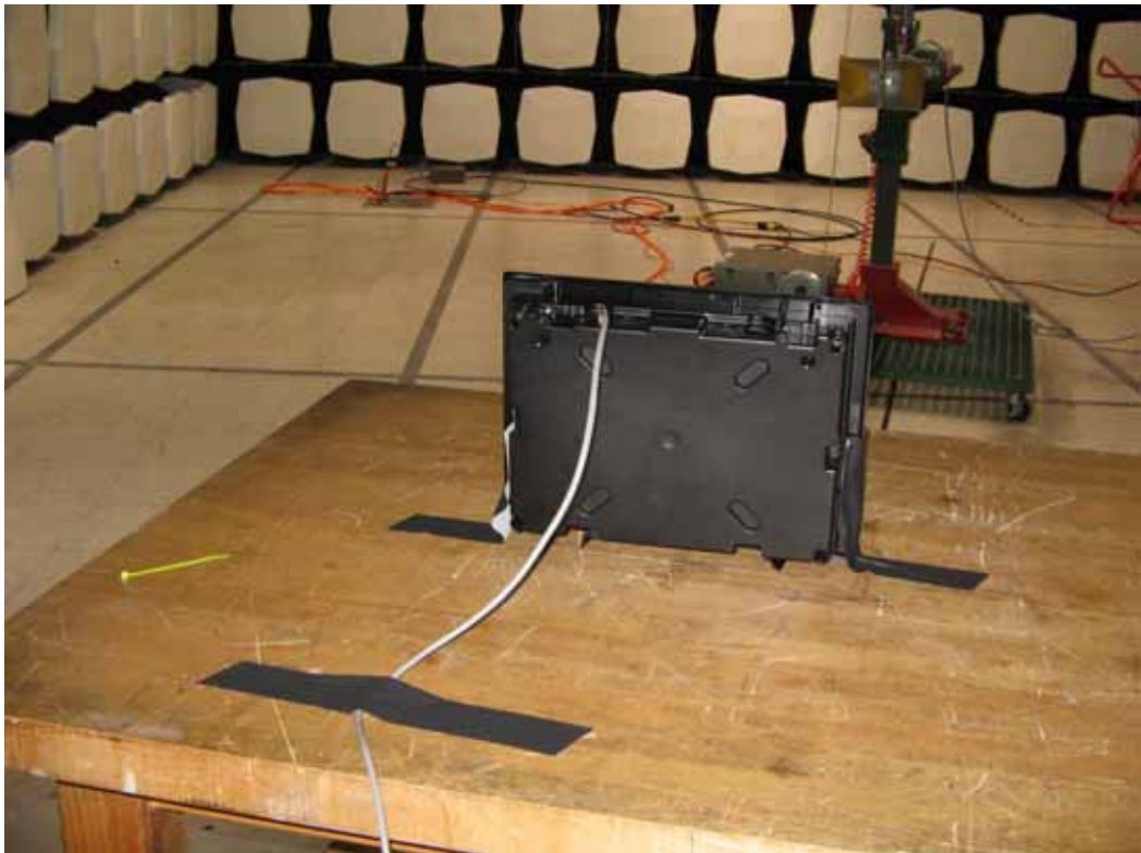
Radiated Emissions Test Configuration – System in the Wall Docking Station
