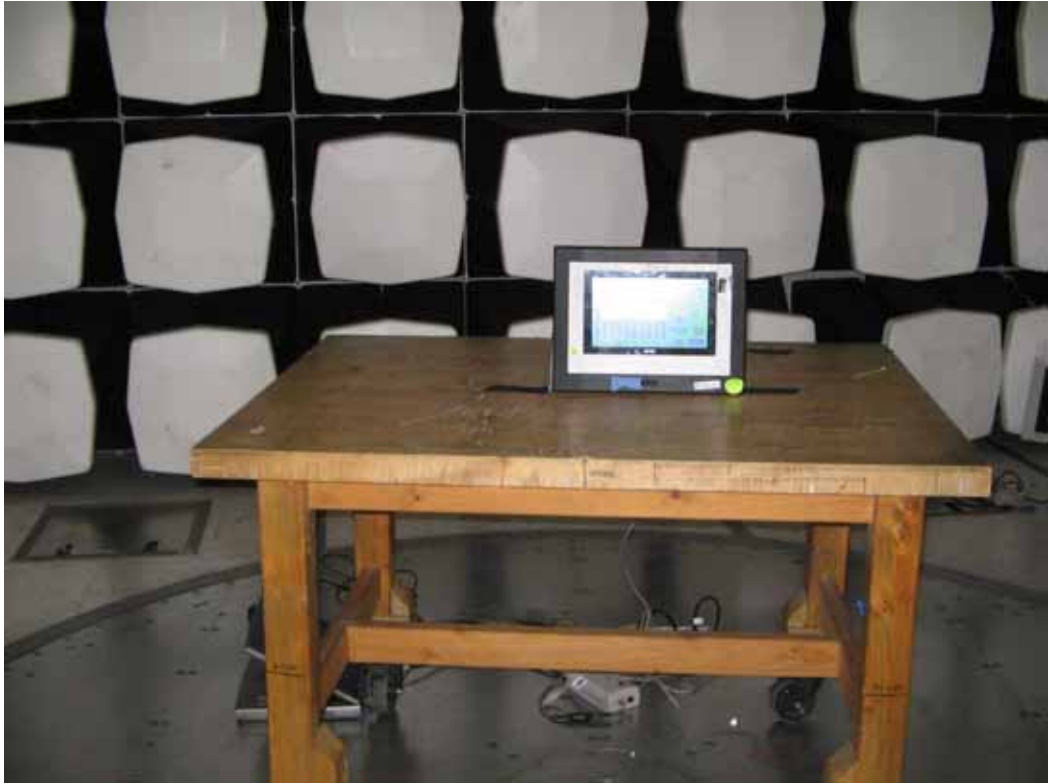
Radiated Emissions Test Configuration – System in the Wall Docking Station
