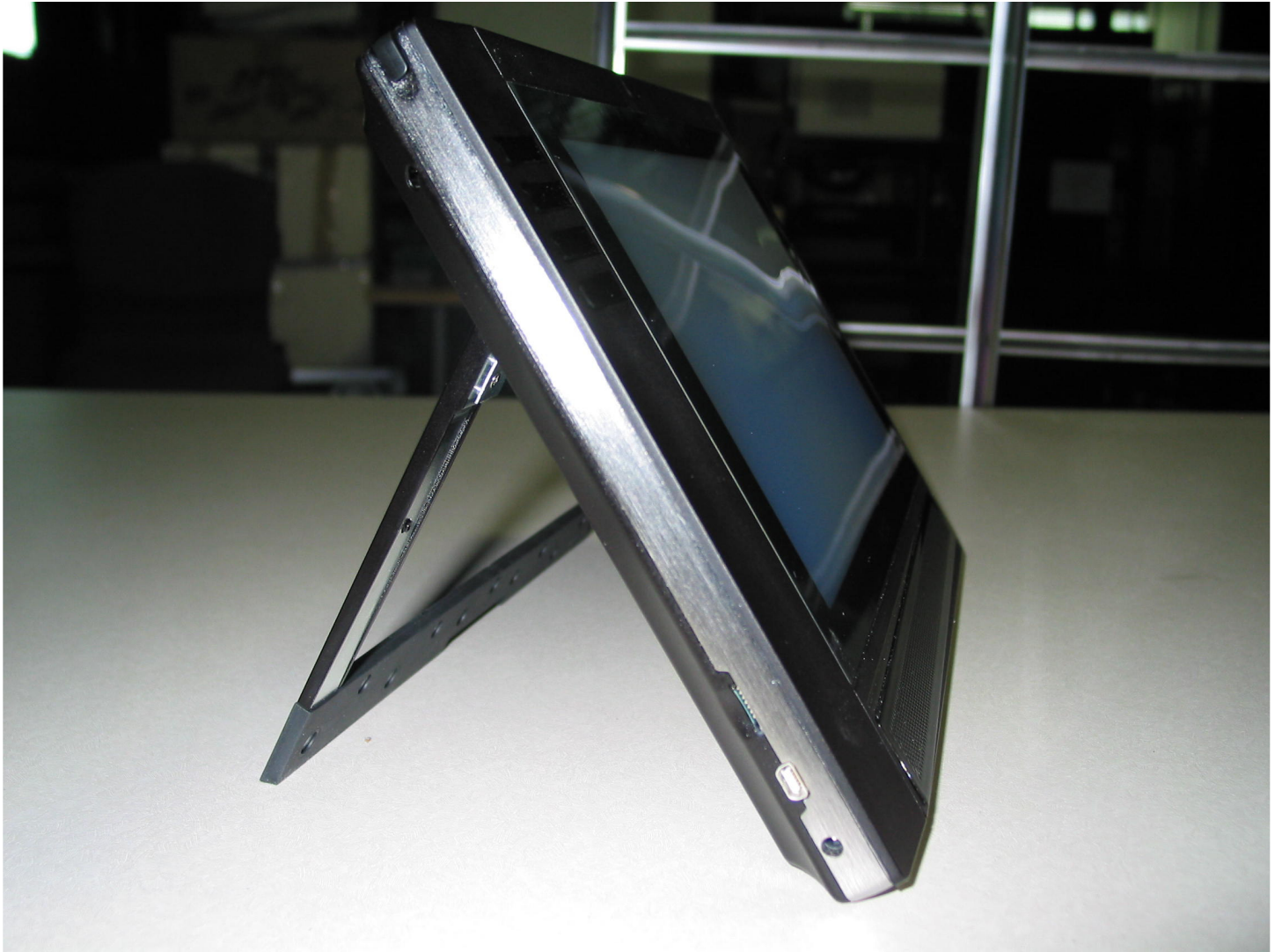
Side of system showing mini USB, USB and power connector
