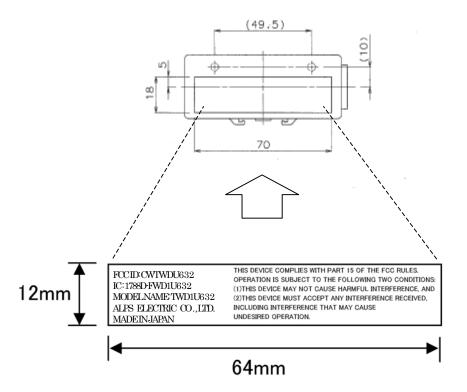
\*The way of attaching FCC ID is "Seal". Material of seal is PET.
