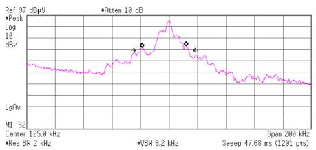
Occupied Bandwidth 30.9335 kHz Occ BW % Pwr 99.00 % x dB -26.00 dB
