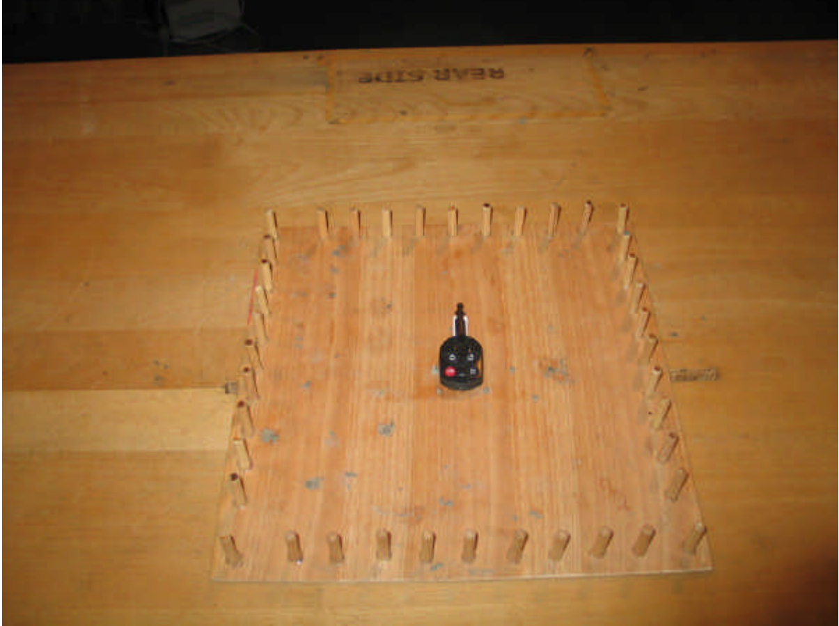
Photo 1: Test setup for radiated measurements
