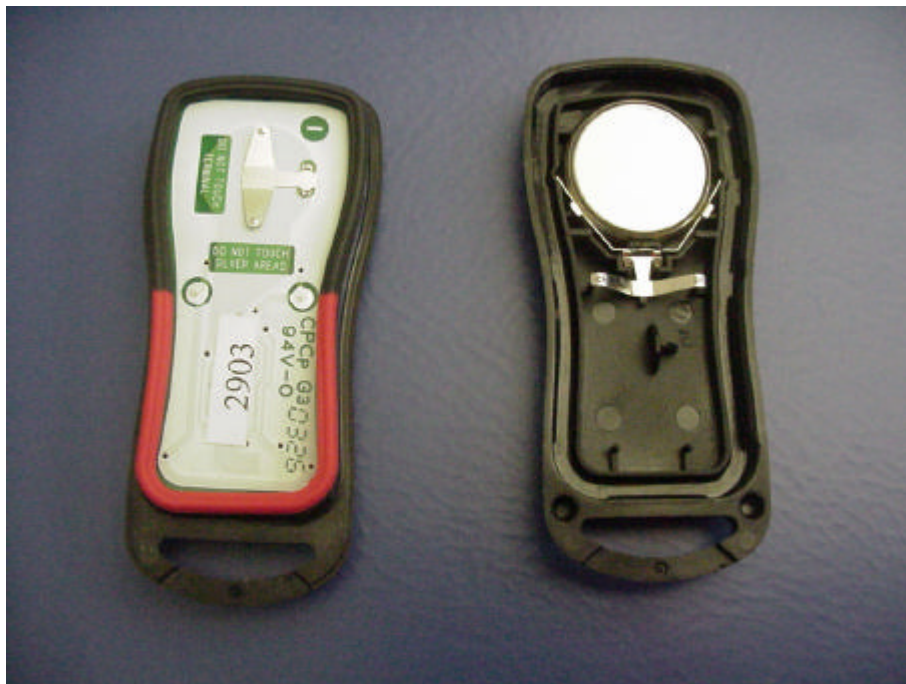
Picture 2 : vehicle remote keyless entry transmitter, inside view
