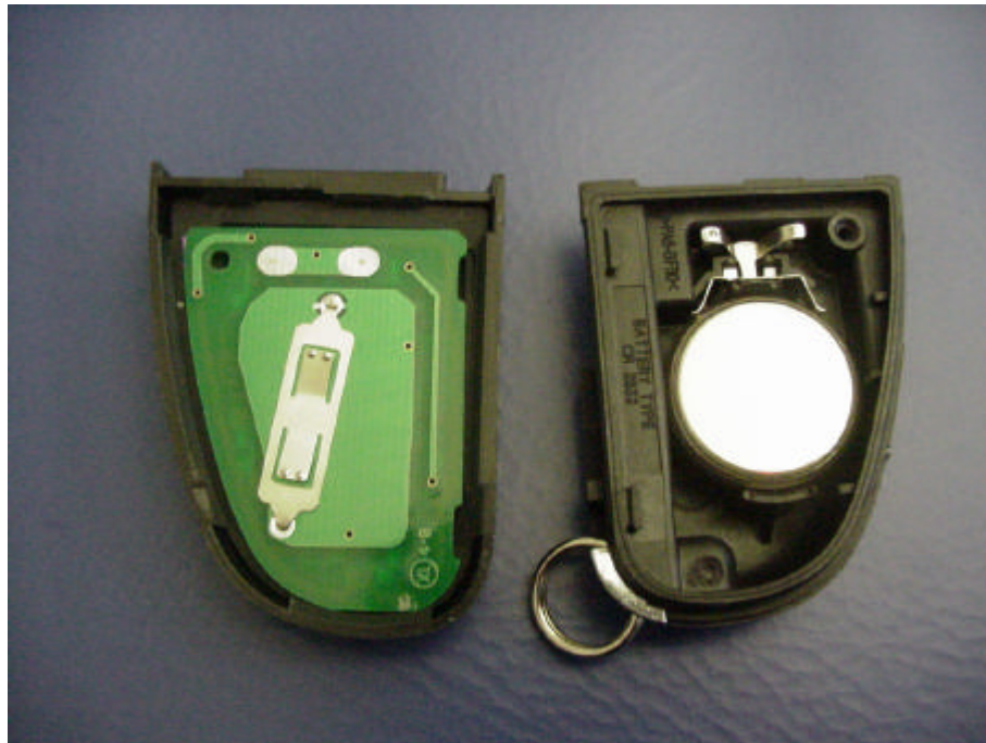
Picture 3 : vehicle remote keyless entry transmitter, inside view
