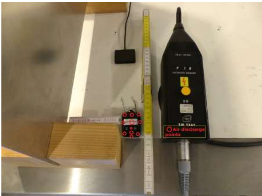
Picture 2 : Setup for the test "ESD" (Air discharge)
