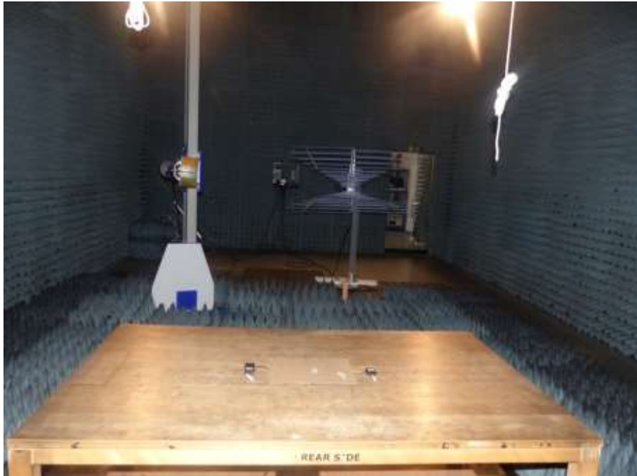
Picture 1 : Setup for the test "RF-electromagnetic field"
