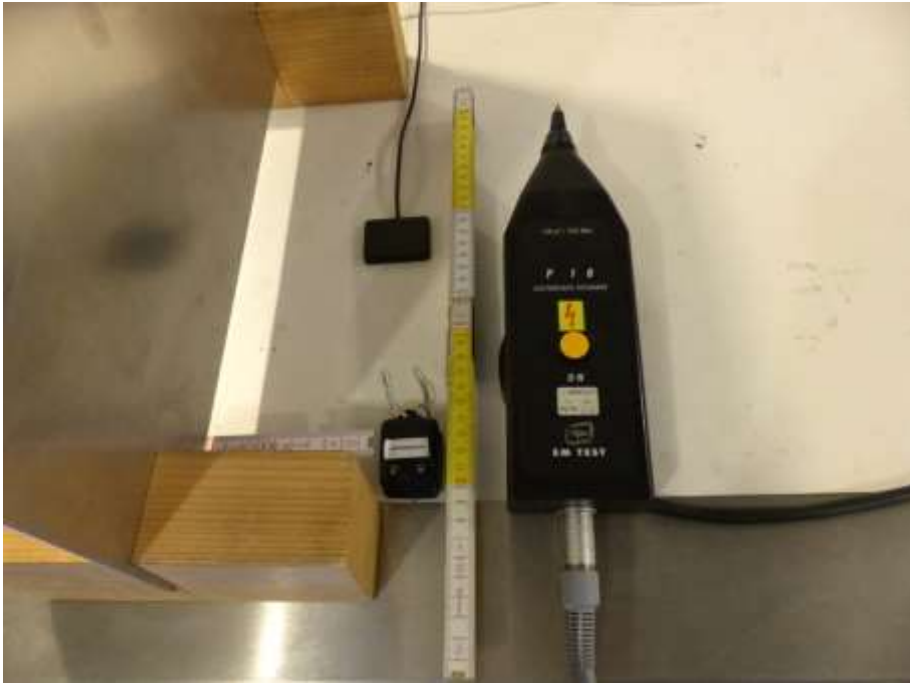
Picture 3 : Setup for the test "ESD" (Indirect and direct ESD)
