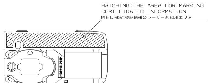
These indications are made inside the product. The user can replace the battery without using any special tool. Users can check their display when replacing the battery.
