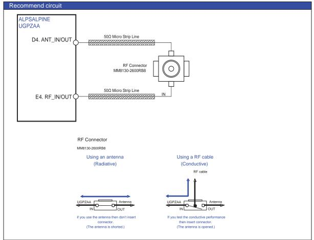
Note: The ground recommend to avoid the ANT pad and to be designed. In addition, the impedance of micro strip line should be use the 50Ω from ANT pad to RF connector, and its length should be shortest connecting. The 50Ω line should be routed on the back of the board on which the module will be mounted. In that case, wire so that it does not overlap the ANT block of the module at the top and bottom.
