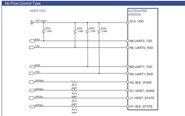
Note: Usually, the ref. R33x (pull-up resister) need. In addition, its resister should be optimizing to the host CPU. The impedance of signal line should be matching to the clock rate.
