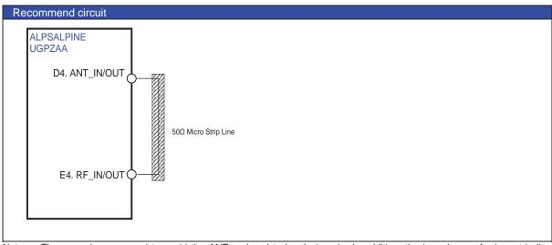
Note: The ground recommend to avoid the ANT pad and to be designed. In addition, the impedance of micro strip line should be use the 50Ω from ANT pad to RF connector, and its length should be shortest connecting. The RF signal line should be surrounded by GND so that it is not affected by external noise.
