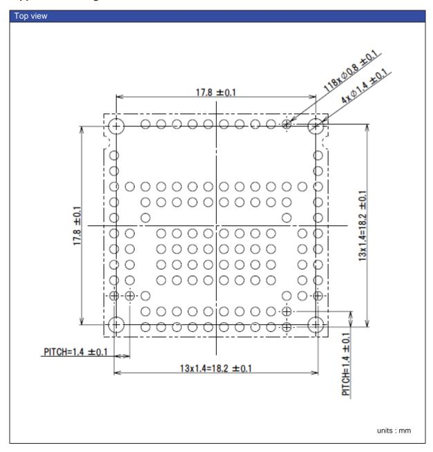
Note: Tolerances are ±0.1mm, unless otherwise specified. Dimensions in (): It is reference dimension.
