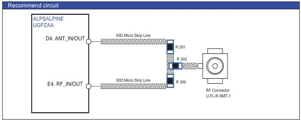
Note: The ground recommend to avoid the ANT pad and to be designed. In addition, the impedance of micro strip line should be use the  $50\Omega$  from ANT pad to RF connector, and its length should be shortest connecting.
