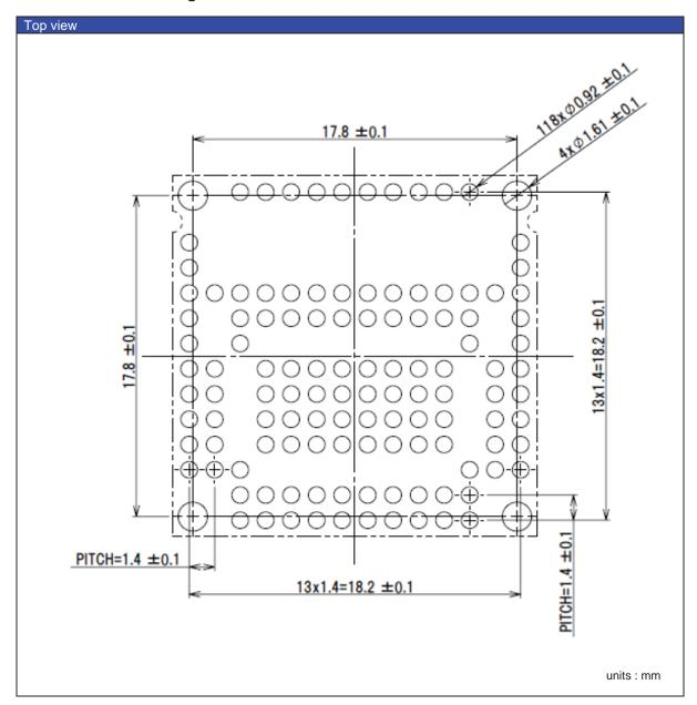
Note: Tolerances are ±0.1mm, unless otherwise specified. Dimensions in () : It is reference dimension. Metal thickness = 0.12 [mm]
