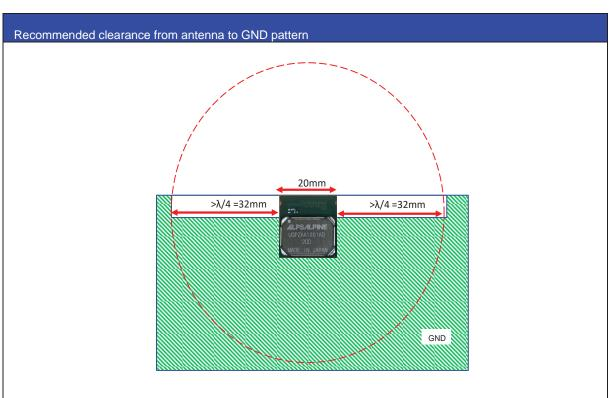
Note: From the antenna to GND, a clearance of 1/4 wavelength or more is desirable. It is desirable that there are no metal parts in the red circle.
