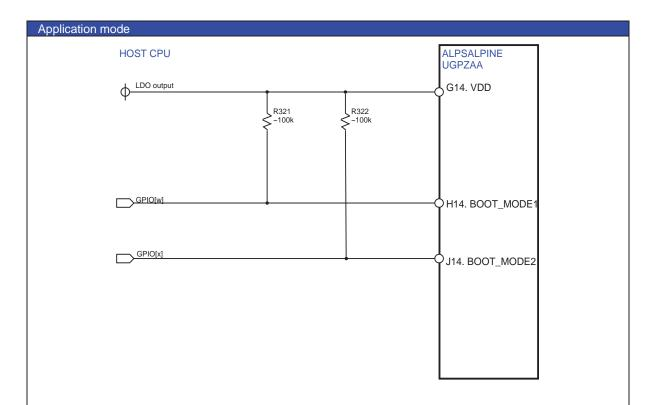
Note: The pins listed in following Table is sampled when RESET\_N de-assert to determine the various operating modes.
